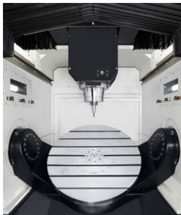
Takumi U 800: Fully enclosed working area
